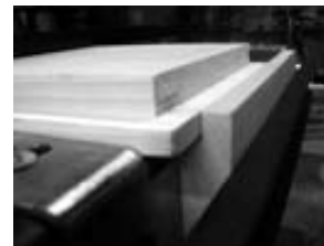
Template removed to show proper positioning of drawer front and gauge block
